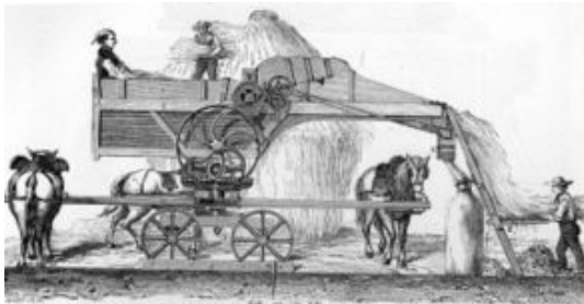
Fig. 318. — Threshing Machine & reaper direct grain into the sack.
