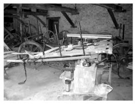
The LM cart was not completed until November 2004 largely because I worked on this one alone. I had to replace much of the upper frame work, the foot well, tail board, part of the floor and part of the shafts. The wheels required a number of The felloes and spokes. metalwork, whilst rusty, was still usable and this is what we have found with all the Carts/Wagons so far. Sandblasting, chemical derust or vigorous wire brushing is usually
