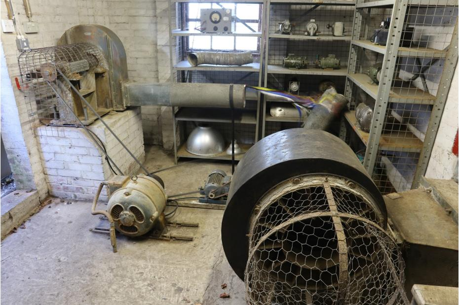
In what was just an old storeroom, one of the major projects has been the installation of the grain silo blower, used to dry the grain. This was one of the first such installations in the country and included an electric heater element installed on the blower outlet at the ducting inlet. You need to come and see this to appreciate all the workings.
