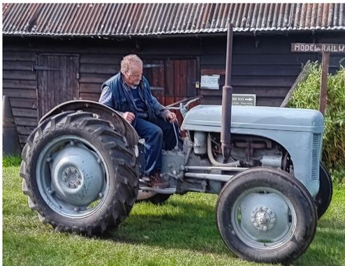
around. The Ferguson System allowed the tractor operator to raise and lower the implement hydraulically from the driver's seat. This system continues to be used on all modern tractors and is the standard throughout the farming world.
